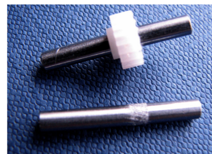
Gear fitted to one axle, with another below to show the knurling by file effect.
