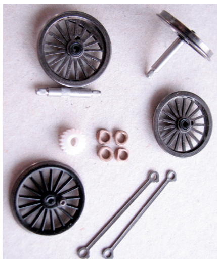
Coupling rods, bushes and gear recovered from original wheels.
