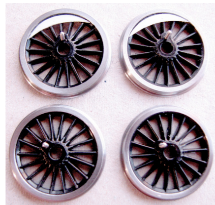
Wheels with crankpins and balance weights fitted.
