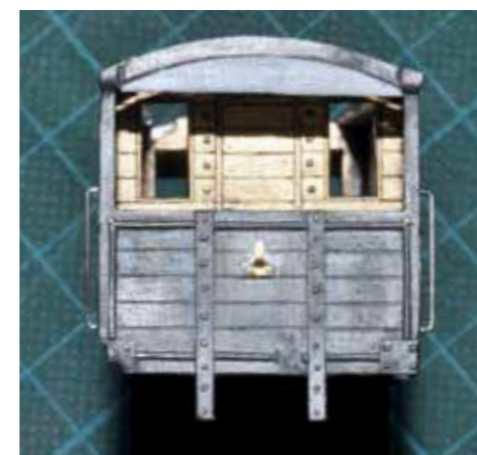
Close up of the cast white metal verandah end prior to painting.
