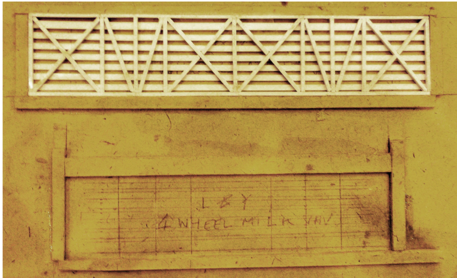
The MDF template with a Diagram 117 side in the upper half, and the guidelines showing in the lower half for the Diagram 111 side.
